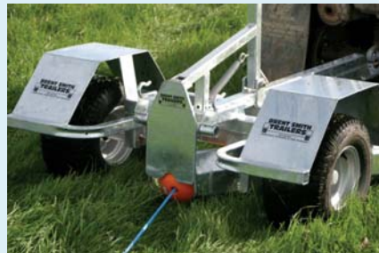
Quick release mechanism allows the shift to be completed without leaving the towing vehicle.
